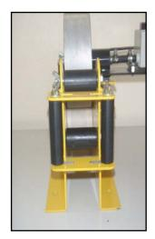
The MU50 is used for the accurate measurement of cable, rope, hose, etc, from 2mm outside diameter up to 50mm. The adjustable guides ensure straight travel of the cable through the meter. The alluminium measuring wheel is directly connected to the re-settable counter and spring loaded to ensure good contact between wheel and cable. The meter can be bench mounted or fitted to a fabricated stand to give a convenient operating height.
